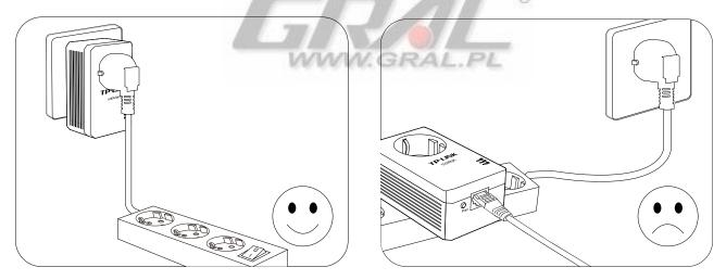
• To take full advantage of the filter function of the Powerline Adapter and to improve data transmission in the network, always plug the multiple sockets into the integrated electrical socket of the Powerline Adapter.
