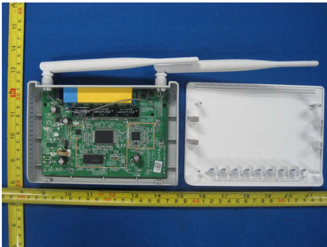
Fig.3 - Internal view of model NBG-418N with non-detachable antenna
