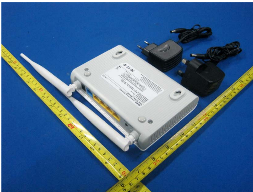
Fig.2 - Overview of model NBG-418N and Power supply (2) (Overall: approx. 163mm x 115mm x 30mm)
